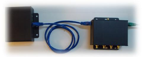
RFtek SmartMux is an antenna multiplexer for UHF RFID applications at 860 – 960 MHz operating frequency with an RF input power of up to 33 dBm (2 Watts). It provides operation up to four antennas with a single antenna input. Especially for multiple antenna applications, it reduces system implementation cost by saving additional readers.
